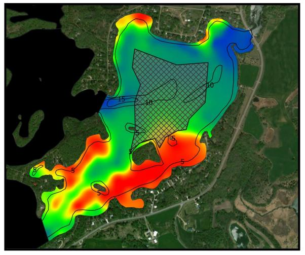
Plant biovolume by sonar and Biobase SAAS. Plant biovolume is the percentage of aquatic plants occupying the water column at a given point. Values of 0 (Blue) indicate no plants and 1 (Red) indicate plants at the surface of the water. Plant volume is not species specific (i.e., it includes more than curlyleaf pondweed). Hatched areas show where sonar data were too poor to generate an estimate or where surveys did not occur.
