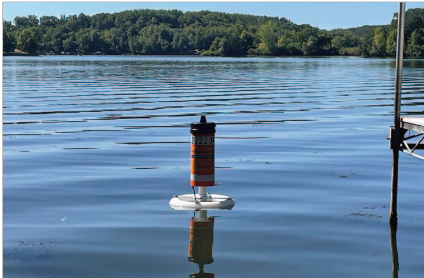
Winter Recreation Technologies has deployed this buoy year-round in Horseshoe Lake to measure water levels.
