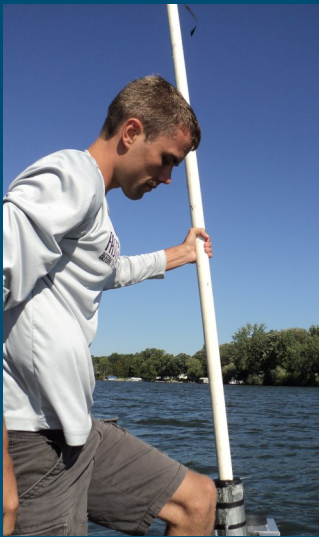
SRWD intern demonstrating the use of a lake surface integrated sampler.
